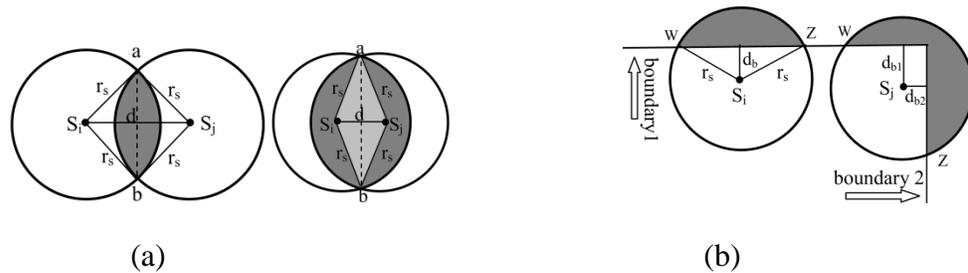
(a) overlapping sensing range neighbors sensors. (b) different positions boundary sensors.
