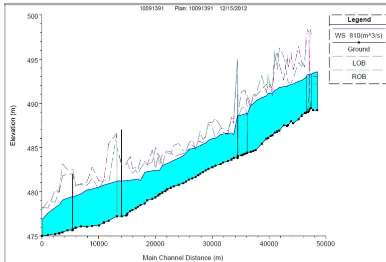
**Figure.5.**River profile of 810 (m<sup>3</sup>/s)
