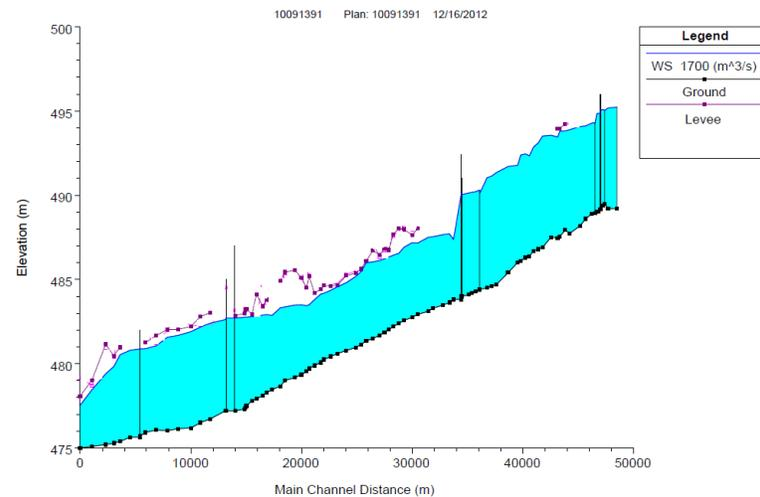
Figure.7.River profile of 1700 (m<sup>3</sup>/s)
