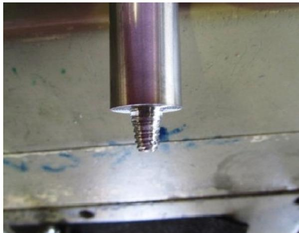
**Figure. 1.** HSS steel tool used for friction stir welding. Shoulder Diameter 20mm, diameter at the bottom of the taper pin: 5.3mm, diameter at the top of the tapered pin: 6.3mm and tool height is 20 mm.
