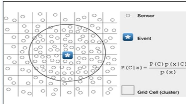
Figure. 5. Setting the sensors in the environment based on the Bayesian Theory.
