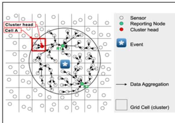
Figure. 6. Divide workspace to grid cells for collecting events by the sensors.
