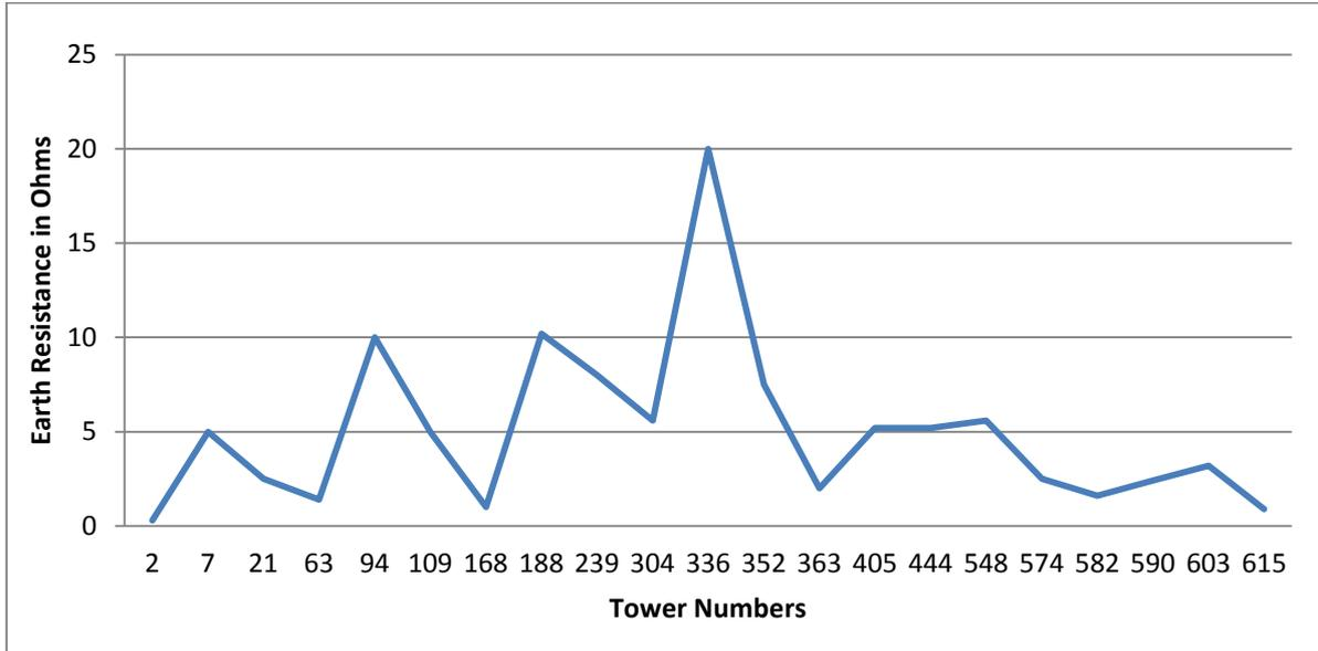
**Figure 3:** Tower Footing Earthing Resistance
