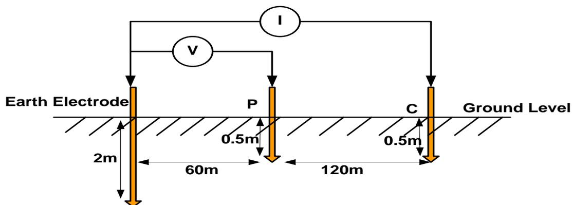
**Figure 2:** Fall-of-Potential Method
