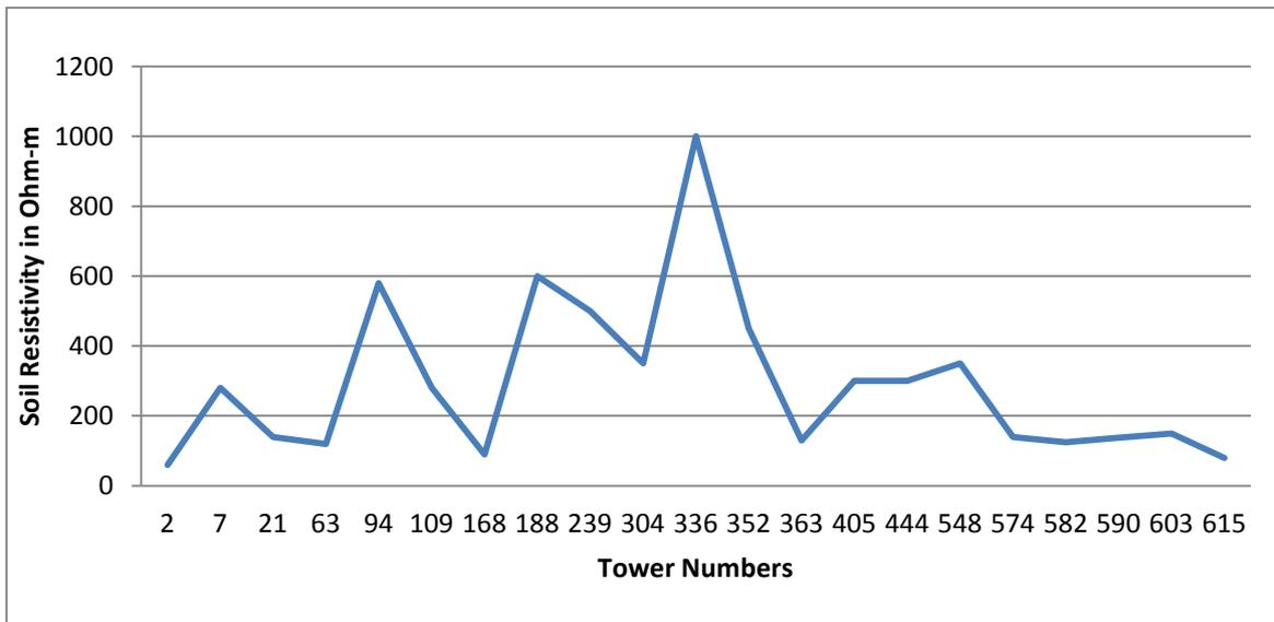
**Figure 4:** Tower Footing Soil Resistivity
